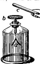
Electroscope. a Gold Leaves made to diverge by repelled electricity due to charged Rod c, an equal and opposite charge being attracted to Cap b.
